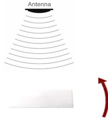
Angular Sensitivity Inlay is rotated in the x,y axis, fixed in z axis )Tag shown at 0° with respect to face of antenna(
