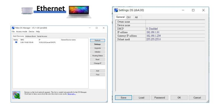
B. Securely insert the Ethernet cable into both the ports of AL-510 and your computer, and revise IP-address to 192.168.1.X. Your AL-510 should be ready by now.
